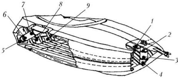
**Figure 2.** Location of characteristic damages of TC: 1 – tip winch strengthening; 2–4 – damages of tip support; 5–7 – places of damages of stern support; 8, 9 – stern strengthening under the engine
