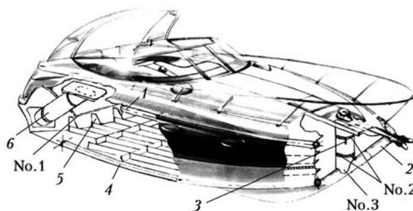
**Figure 1.** Scheme of welded structure of TC hull of alloy AMg6: 1 – strengthening of deck; 2 – tip tail of keel; 3 – tip support; 4 – bottom strengthening; 5 – knee; 6 – stern support; No.1 – stern strengthening weld; No.2 – support weld; No.3 – weld of support fastening at the stem
