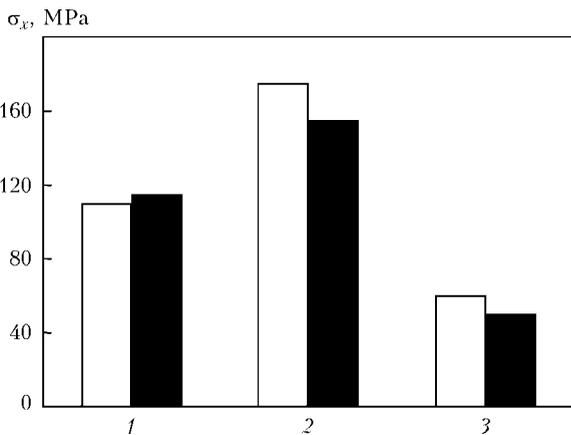
**Figure 3.** Longitudinal RS in the specimens of longitudinal (white columns) and circumferential (black) welds: 1 – initial RS; 2 – after repair welding; 3 – after EDT
