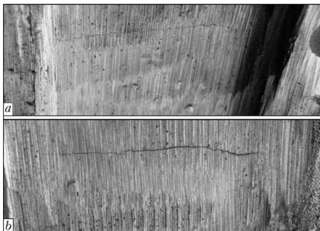
**Figure 9.** High-temperature cracking of circumferential welds in zone of joint of flange (steel 15Kh5MU) to heat exchanger shell (12KhM) of various thickness: *a* – weld joining heat exchanger shell to bottom of 35 mm thickness; *b* – weld in the zone of joint of 45 mm thickness shell to flange
