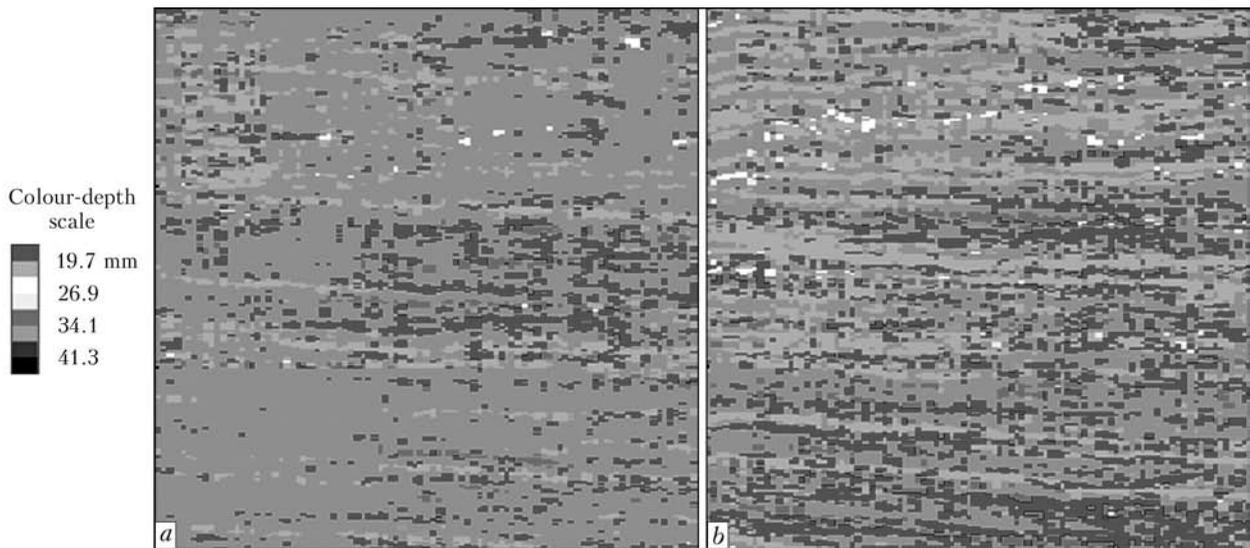
**Figure 3.** Monitoring of growth of discontinuities in the metal of absorber body from 09G2S steel of 48 mm thickness during one year of operation (reference section of 750 × 750 mm size): *a* – initial scanning; *b* – repeated scanning of the same section after one year
