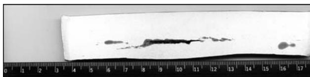
Figure 2. Lamellar cracking across sheet thickness
