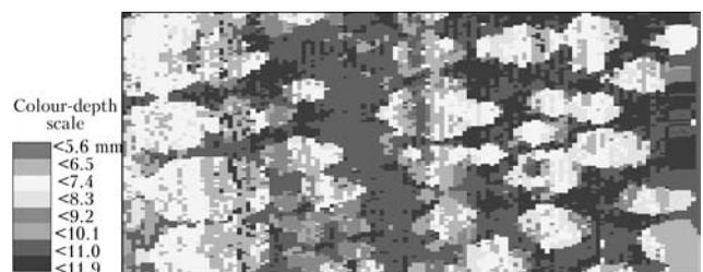
**Figure 5.** Fragment of scanned section with hydrogen cracking of an element of absorber body from St3sp5 steel 12 mm thick (section size of 250 × 250 mm)
