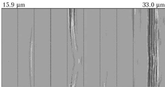
**Figure 10.** Example of TOFD measurement of a crack in a welded joint which initiated through cracking of facing cladding layer
