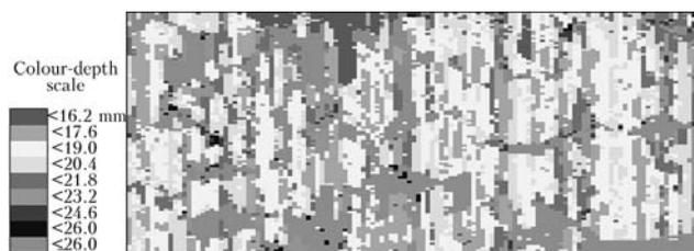
**Figure 4.** Data on scanning in section of absorber case from 16GS steel 28 mm thick (section size of 250 × 500 mm)
