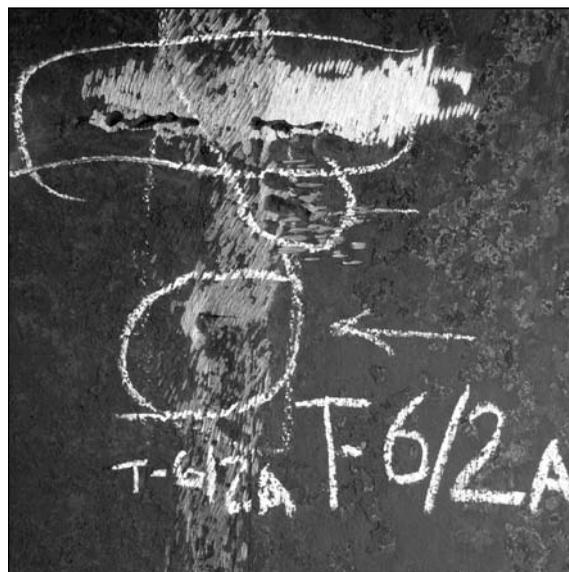
**Figure 8.** High-temperature cracking of weld of heat-exchanger from 12KhM steel in repair welding zone
