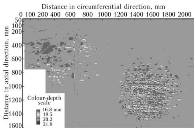
**Figure 6.** Data of scanning in the section of column body opposite to product input (MEA water solution) (section size of  $1600 \times 2000$  mm, metal thickness of 22 mm)
