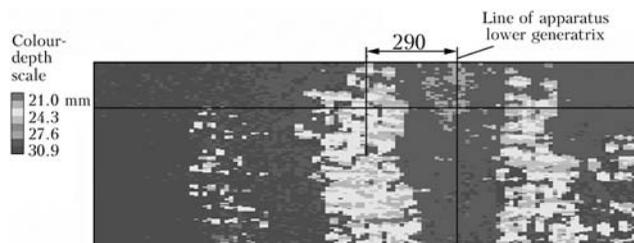
**Figure 7.** Data on scanning metal with corrosion damage in stagnation zone of separator 32 mm thick from steel 16GS (section size of  $500 \times 1750$  mm)
