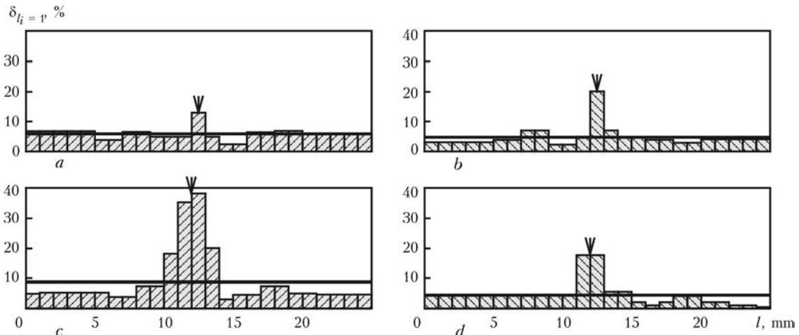
**Figure 6.** Character of distribution of residual elongation in tensile tests of butt joints brazed with the Cu-Ti system filler metal in vacuum furnace by using radiation heating (*a* – specimen No.3; *b* – No.4), and by the flowing current (*c* – No.13; *d* – No.14):  $\delta_{2.5} = 5.90$  (*a*), 4.76 (*b*), 8.86 (*c*) and 4.35 (*d*) %
