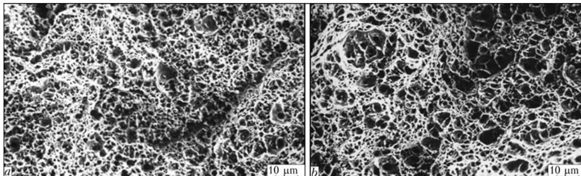
Figure 2. Fractographs of fracture surface of base metal in initial state (*a*) and after annealing (*b*)
