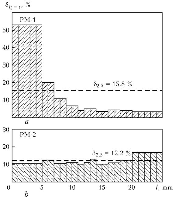
Figure 3. Character of distribution of residual elongation in tensile tests of cylindrical specimens of alloy Glidcop Al-25 in initial state (a) and after annealing (b)
