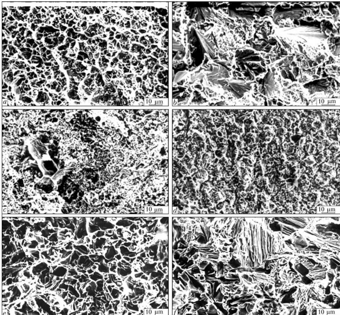
Figure 4. Fractographs of fractures of brazed joints on dispersion-strengthened copper alloy produced with filler metals Nos. 4 (a), 3 (b), 2 (c, d) and 1 (e, f)
