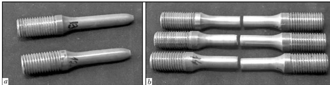
Figure 1. Appearance of specimens after mechanical tests: *a* – base metal; *b* – brazed joints
