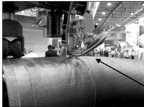
Figure 8. Working body of the following system mounted on the welding head
