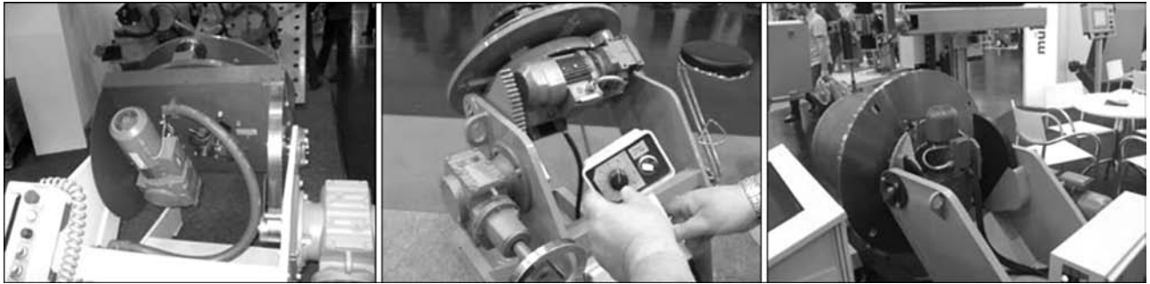
Figure 1. All-purpose manipulators with asynchronous electric motor in the rotation drive
