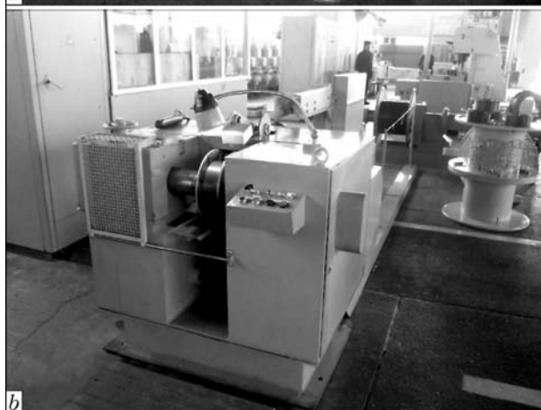
Automatic line on manufacture of flux-cored wire (forming, filling, drawing) (a) and installation for coiling of flux-cored wire on framed spools K-300 (BS-300) (b)
