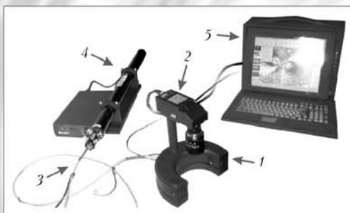
At the E.O. Paton Electric Welding Institute a compact measuring system and technology for determination of residual stresses, occurring in welded, brazed, cast and other metallic structures, have been developed. The developed system and technology can be also used for determination of stresses, caused in structures by applying the loads.
