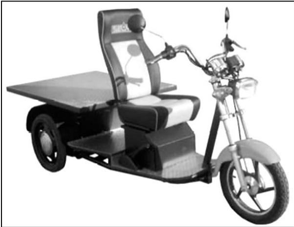
The electrocycle is a three-wheel electric vehicle equipped with a handle bar, one front guide wheel and two rear guide wheels.
