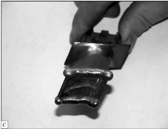
Figure 6. Geometric characteristics of repair zone ( a , b ) and appearance ( c ) of repaired HPT blade of alloy JS32-VI: \square , \circ – 1.0 and 2.5 mm decrease, respectively, in thickness of the damaged surface prior to cladding in a batch of N = 100 blades; \delta – width of flange platform face
