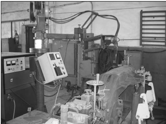
Figure 4. Experimental-industrial setup for hardfacing of guide surfaces of axle box opening of side frame of truck of the 18-100 model freight car
