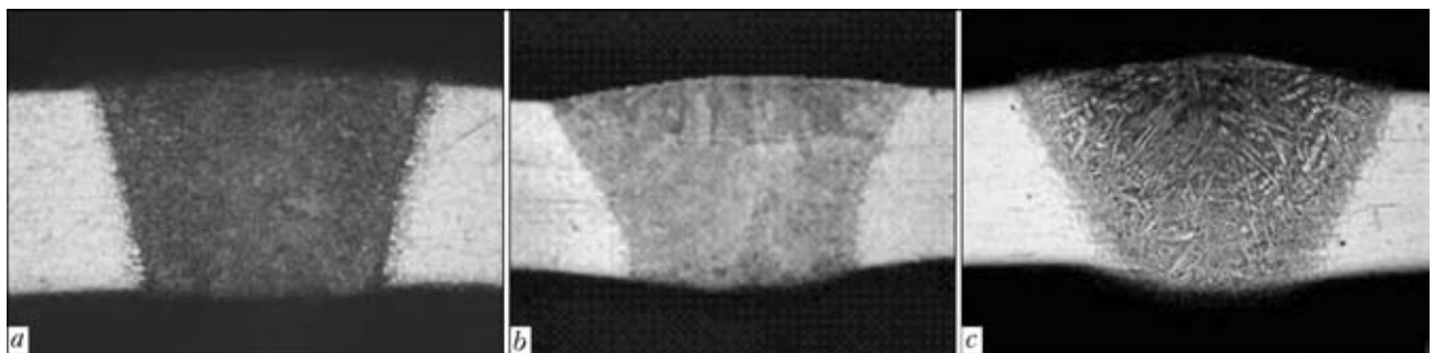
Figure 2. Macrosections ( \times 20 ) of butt welded joints produced by orbital EBW in two passes: a – steel 304SS; b – titanium alloy PT-3V; c – monel alloy
