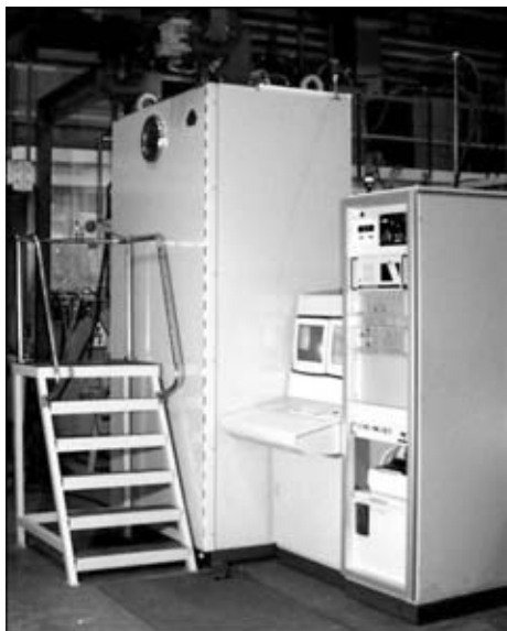
Figure 8. Appearance of specialized system UL-178M for EBW of tubes to tubesheets
