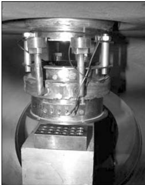
Figure 2. Appearance of deflection system with double refraction of the electron beam mounted on electron beam gun ELA-60/15
