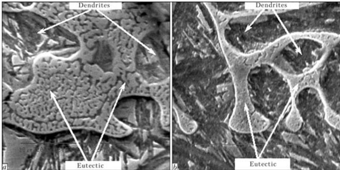
**Figure 4.** Microstructures ( $\times 9600$ ) of fusion zone between steel St3 and high-chromium cast iron illustrating dendritic-eutectic structure produced without (a) and with LRO (b)
