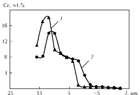
**Figure 5.** Dependence of content of chromium in fusion zone upon cladding parameters: 1 – without LRO; 2 – with LRO;  $l$  – distance from fusion line
