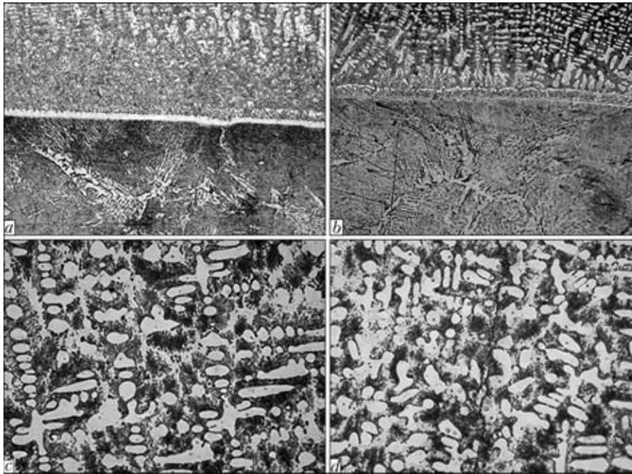
**Figure 2.** Microstructures of fusion zone between steel St3 (*a, b* –  $\times 400$ ) and deposited high-chromium cast iron (*c, d* –  $\times 1000$ ) obtained without (*a, c*) and with LRO (*b, d*)
