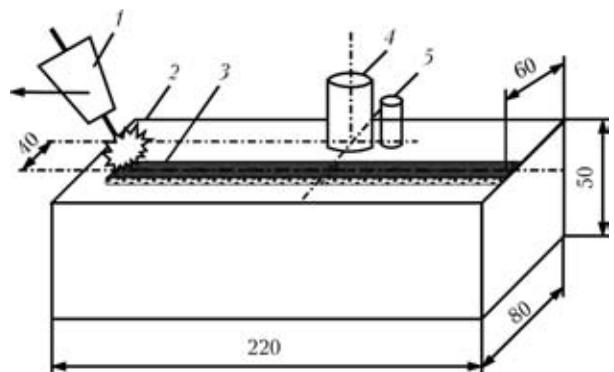
Figure 1. Flow diagram of cladding of samples by involving the external effect by LRO: 1 – welding head; 2 – sample; 3 – deposited cast iron bead; 4 – oscillations exciter; 5 – sensor
