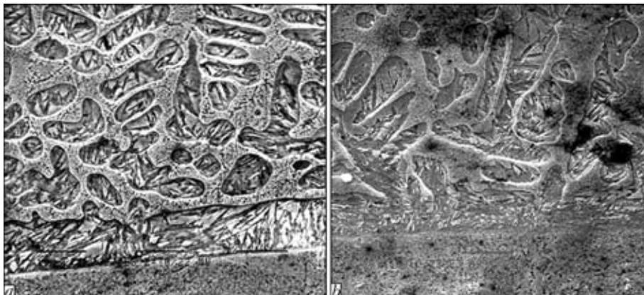
**Figure 3.** Microstructures ( $\times 2300$ ) of high-chromium cast iron fusion zone obtained without (*a*) and with LRO (*b*) under scanning electron microscope
