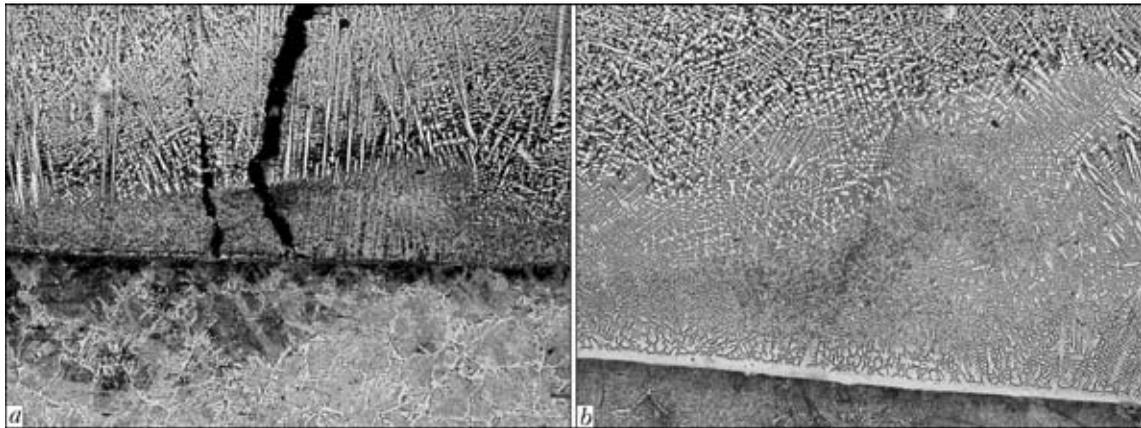
**Figure 6.** Microstructures ( $\times 300$ ) of typical sites of initiation of cracks in deposited high-chromium cast iron produced without (a) and with LRO (b)
