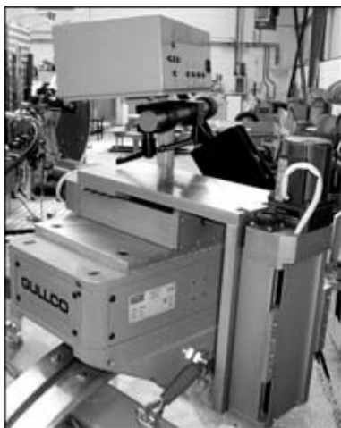
Figure 4. Gullco orbital system for welding pipes
