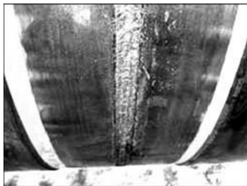
Figure 1. Cover pass of weld on a pipe in manual arc welding
