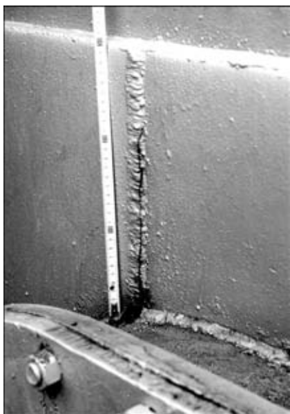
Figure 2. Crack propagation in the circumferential weld made on reinforcing coverplate of the oval hatch in the oil tank of 20,000 m 3 capacity from 09G2S-12 steel with 16 mm wall thickness
