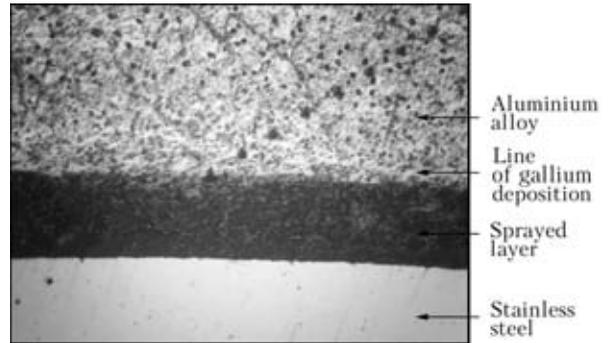
Figure 3. Microstructure (x300) of the zone of joining with dents of Berkovich indenter
