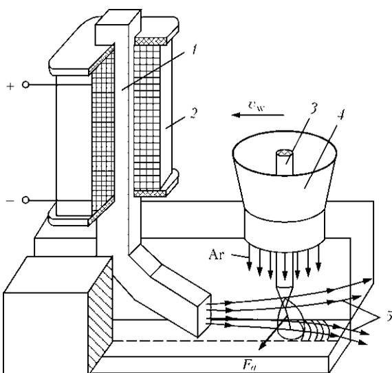
**Figure 1.** Flow diagram of NGW with controlling magnetic field: 1 – electromagnet core; 2 – electromagnet coil; 3 – tungsten electrode; 4 – protective nozzle; 5 – force lines of controlling magnetic field
