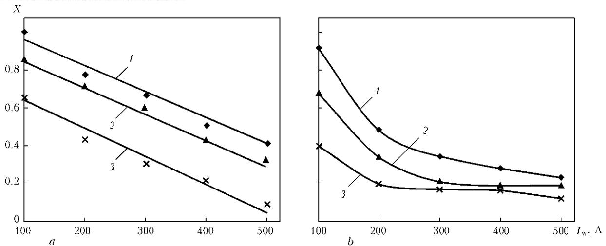
Figure 7. Dependence of the fraction of the current flowing through the side wall on the welding current when using electrodes with flat (a) and cone-shaped (b) tips: 1 –  $B_x = 11.4$ ; 2 – 10.1; 3 – 6.1 mT
