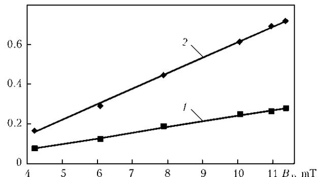
**Figure 6.** Dependence of the fraction of the current in a side wall of the groove on magnetic induction  $B_x$  when using tungsten electrodes with cone-shaped (1) and flat (2) tips ( $I_w = 400$  A)
