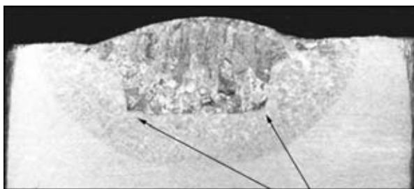
**Figure 3.** Macrosection of the deposited metal with lack of penetration at the groove corners (material – titanium alloy PT3V, filler wire VT1-00)
