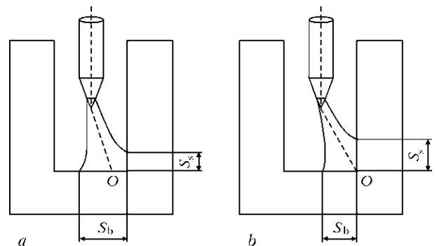
**Figure 5.** Schematic of location of the anode spot at insufficient (*a*) and optimal (*b*) deflection of the arc in the groove:  $S_b$ ,  $S_s$  – distances from the centre of the anode spot at the bottom and side walls, respectively
