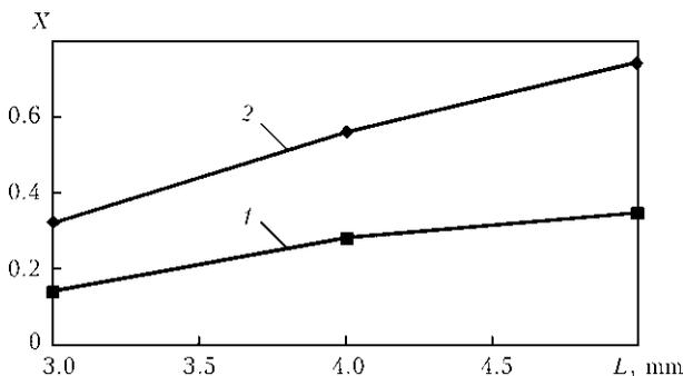
Figure 8. Dependence of the fraction of the current in a side wall of the groove on arc gap length  $L$  when using electrodes with cone-shaped (1) and flat (2) tips at  $B_x = 11.5$  mT and  $I_w = 400$  A
