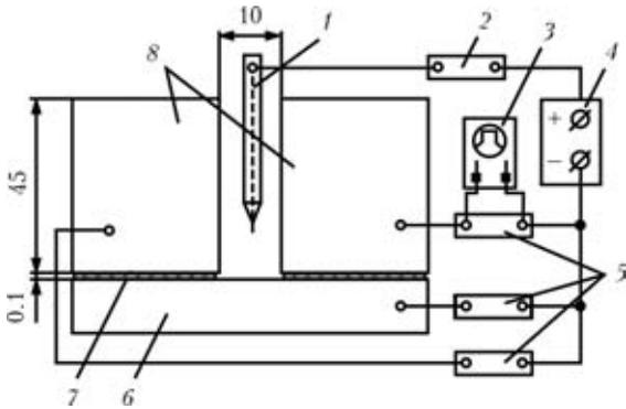
**Figure 2.** Scheme of the unit to measure the current flowing through the side walls of the groove in NGW with the controlling magnetic field: 1 – tungsten electrode; 2 – shunt to measure the welding current; 3 – oscillograph; 4 – power supply; 5 – shunts to measure the welding current flowing through the side and bottom walls; 6 – bottom wall of the groove; 8 – side walls
