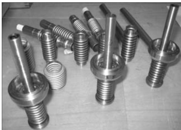
Figure 6. Samples of multilayer bellows manufactured by laser welding of tubular billets of steel 1.4541 with \delta = 0.15 \text{ mm}
