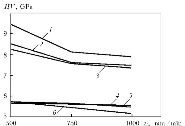
**Figure 6.** Dependence of coating surface layer hardness on parameters of laser cladding mode for materials of Ti-Si (1-3) and Ti-NiCr (4-6) systems: 1, 6 –  $v_n = 6000$ ; 2, 5 –  $v_n = 4500$ ; 3, 4 –  $v_n = 3000$  rpm
