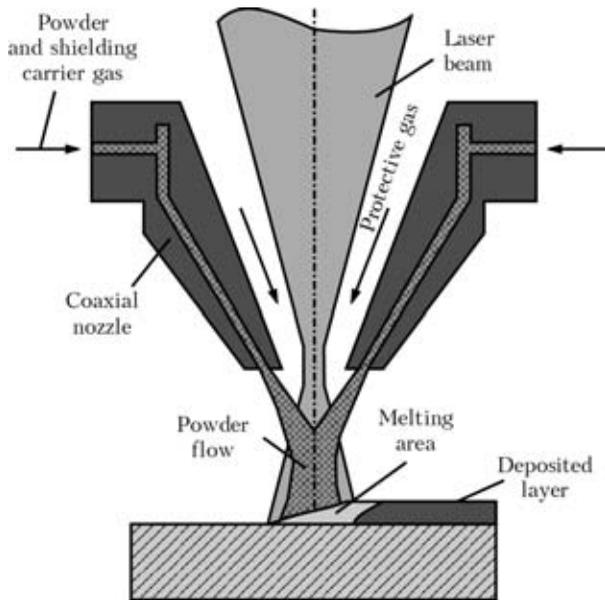
Figure 2. Schematic of laser cladding
