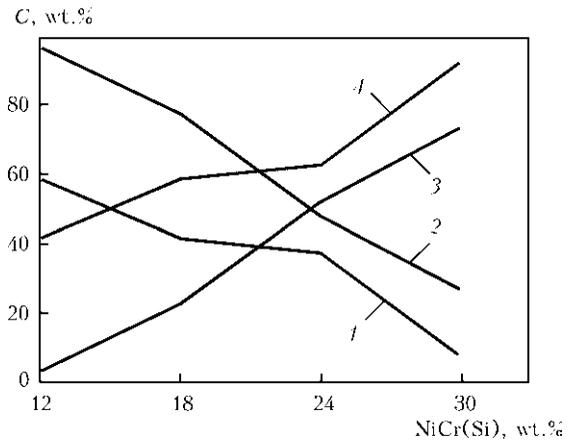
Figure 4. Influence of the content of NiCr(Si) alloying component on phase composition of materials of Ti–Si and Ti–NiCr systems: 1 –  $\alpha$ -Ti; 2 –  $\beta$ -(Ti–Cr); 3 –  $\text{NiTi}_2$ ; 4 –  $\text{Ti}_3\text{Si}_3$
