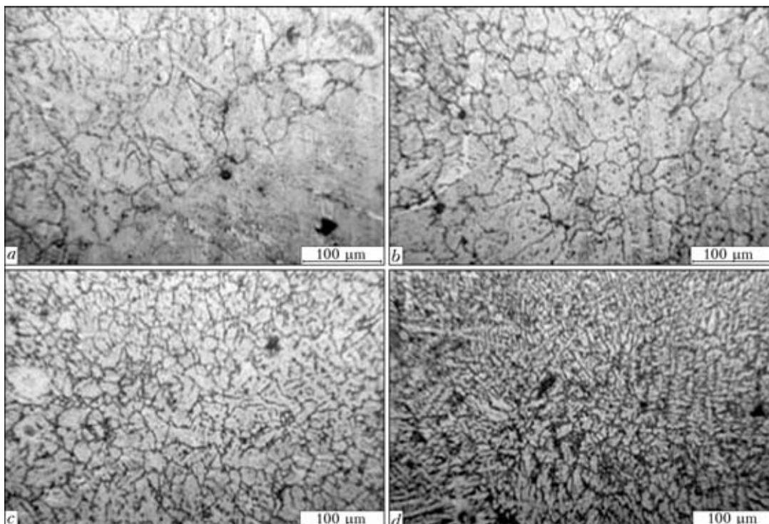
Figure 3. Microstructures of the deposit of Ti–NiCr system material from the substrate to the subsurface layer: a – first layer, 12 wt.% NiCr; b – second layer, 18 wt.% NiCr; c – third layer, 24 wt.% NiCr; d – fourth layer without NiCr
