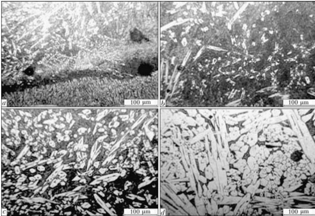
**Figure 5.** Microstructures of deposit of Ti-Si system material from the substrate to subsurface layer: *a* – first layer with 12 wt.% Si; *b* – second layer with 18 wt.% Si; *c* – third layer with 24 wt.% Si; *d* – fourth layer with 30 wt.% Si
