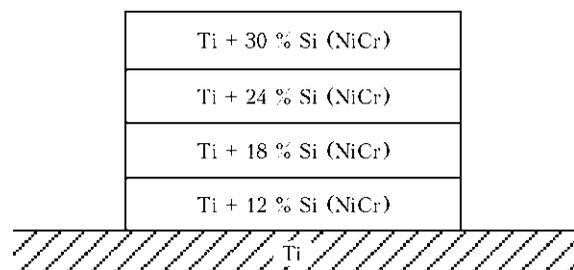
**Figure 1.** Schematic of the change of layer composition by height of deposit of Ti-Si and Ti-NiCr system coatings
