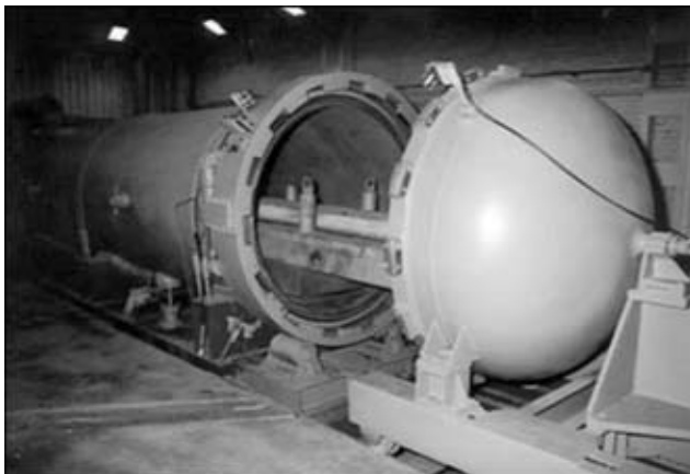
Figure 1. Explosion chamber KVG-16 with pulled out work table
