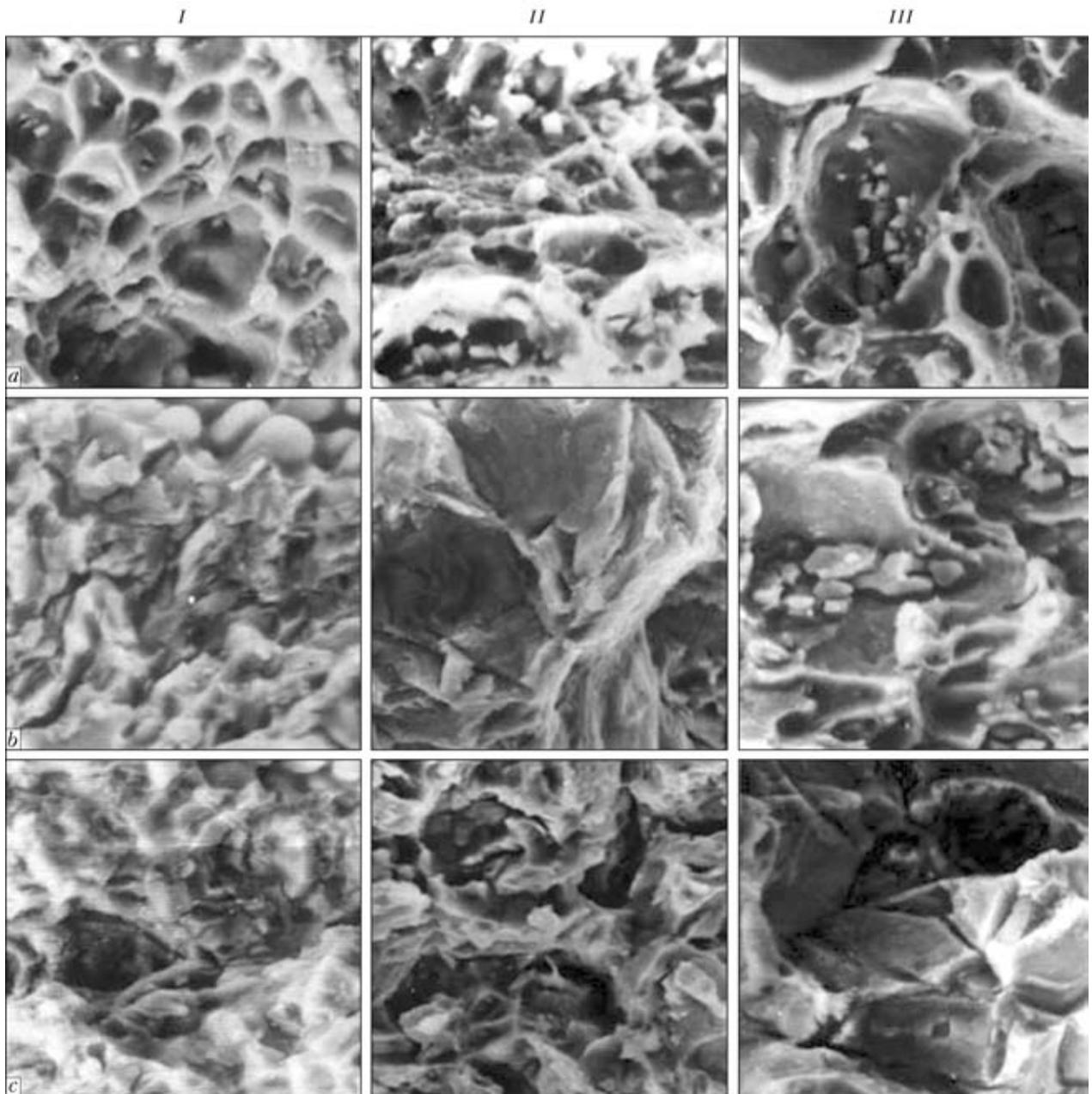
**Figure 4.** Fractograms of fracture surface of individual zones of 1201 alloy welded joint at low testing temperature (*a-c* and *I-III* – see Figure 3)
