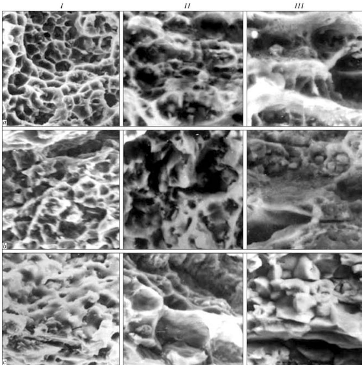
**Figure 3.** Fractograms of fracture surface of individual zones of welded joint of AMg6N alloy tested at the temperature of 293 (a), 77 (b) and 20 (c) K: I – W; II – FZ; III – HAZ
