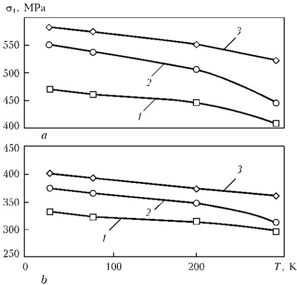
**Figure 1.** Influence of low-temperatures on ultimate tensile strength  $\sigma_t$  of notched samples of aluminium alloys AMg6N (1), 1201 (2) and 1460 (3) (a) and their welded joints (b)
