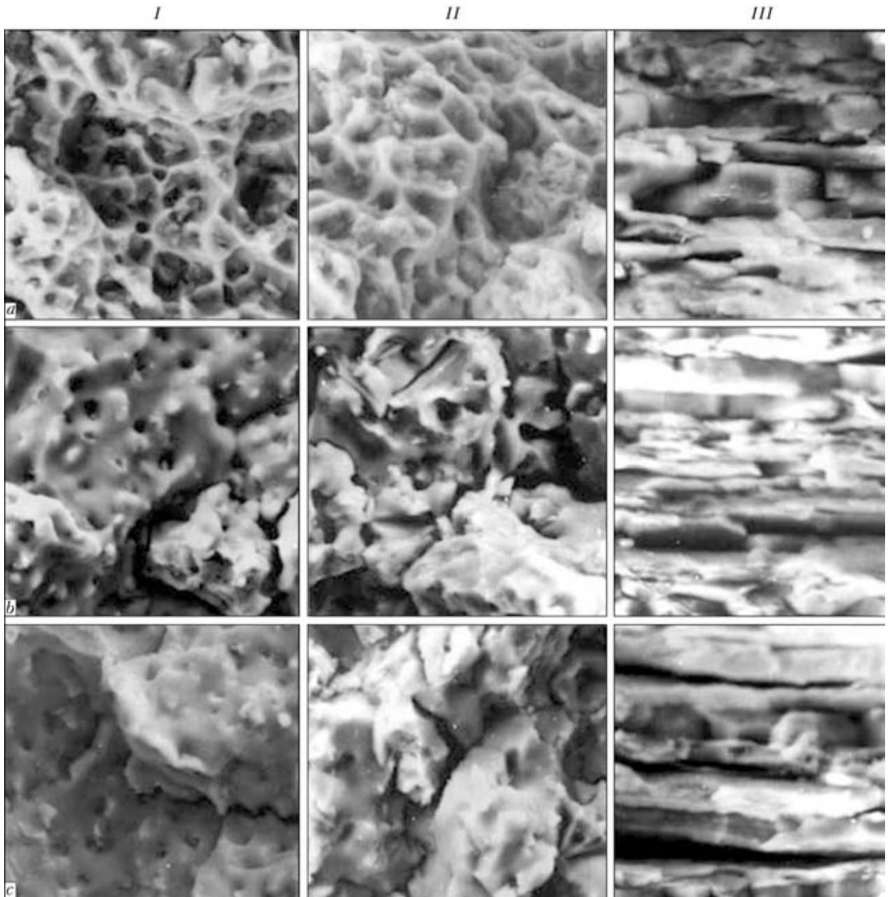
**Figure 5.** Fractography of fracture surface of individual zones of 1460 alloy welded joint at low testing temperature (*a-c* and *I-III* – see Figure 3)
