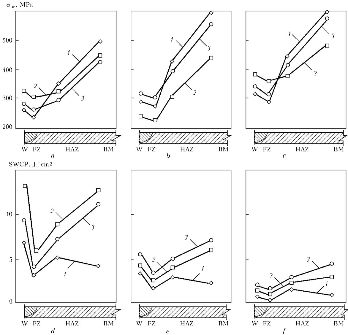
**Figure 2.** Dependence of nominal breaking stress  $\sigma_{br}$  (a-c) and SWCP (d-f) in different zones of welded joints of high-strength aluminium alloys 1460 (1), AMg6N (2) and 1201 (3) on testing temperature of 293 (a, d), 77 (b, e) and 20 (c, f) K: W – weld; FZ – fusion zone; BM – base metal
