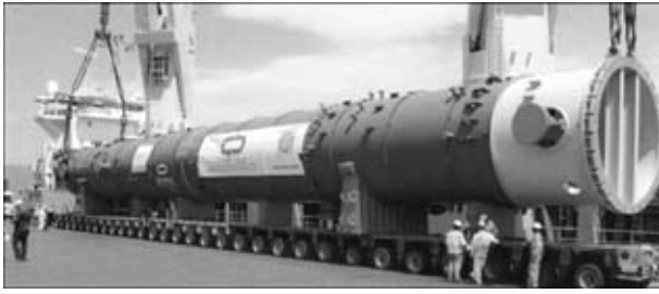
Figure 9. Loading of a 500 t slug catcher surge vessel onto a freighter at Gemlik harbour
