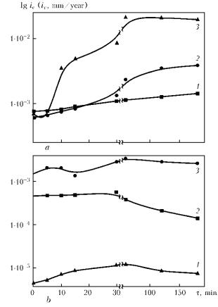
**Figure 2.** Kinetics of corrosion rate  $i_c$  on structural steel St3 under conditions simulating the atmospheric ones with (*a*) and without (*b*) moisture condensation on the metal surface at T = 24 (1), 50 (2) and 70 (3) °C, which was determined with the help of the corrosion rate sensor
