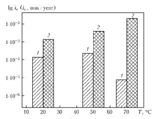
**Figure 4.** Dependence of  $i_c$  of structural steel St3 on temperature under conditions simulating the atmospheric ones with (1) and without (2) moisture condensation on the sensor surface, determined by using the corrosion rate sensor
