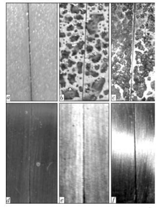
**Figure 3.** Appearance of the surface of sensors after exposure (t = 3 h) to conditions simulating the atmospheric ones with (a-c) and without (d-f) moisture condensation on the sensor surface at T = 24 (a, d), 50 (b, e) and 70 (c, f) °C
