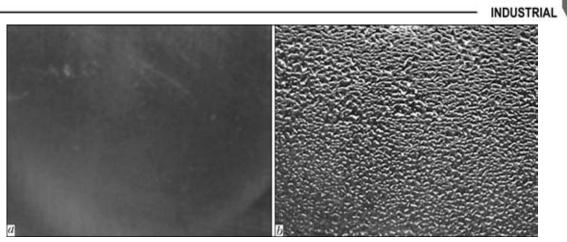
**Figure 1.** Appearance of the moisture film formed on the surface of steel St3 and its welded joints at T = 24 °C without moisture condensation (*a*) and at T = 50 °C with moisture condensation (*b*)
