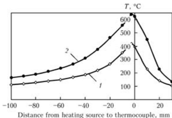
Figure 5. Distribution of temperature in longitudinal direction at the distance of 5 mm from the weld axis in FSW (1) and TIG welding (2) of butt joints of AMg5M alloy
