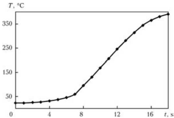
**Figure 1.** Distribution of temperature of heating of AMg5M alloy at the distance of 6 mm from the weld centre in FSW at  $v_w = 8$  m/h at deepening of working tool with 12 mm diameter shoulder and tip of conical shape
