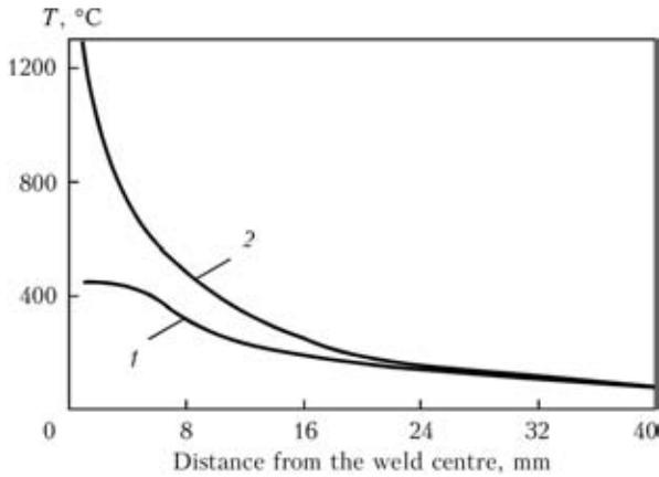
Figure 4. Distribution of temperature in transverse direction of butt joints of AMg5M alloy produced using FSW (1) and TIG welding (2)
