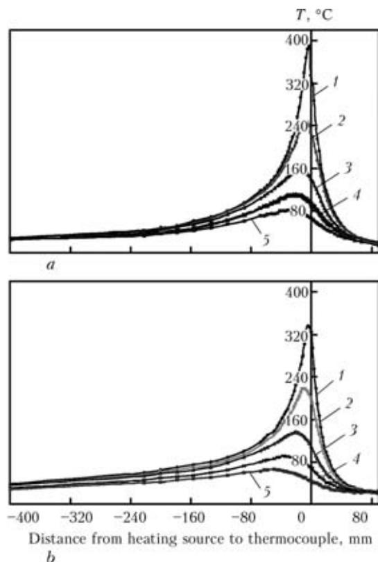
**Figure 3.** Distribution of temperature in FSW of AMg5M alloy butt joint at  $v_w = 8$  (a) and 20 (b) m/h and different moving from the weld axis: 6 (1), 11 (2), 21 (3), 31 (4) and 40 (5) mm
