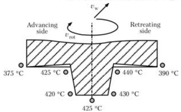
**Figure 2.** Temperature points of metal in the FS-welded joint on AMg5M alloy at  $v_w = 8$  m/h
