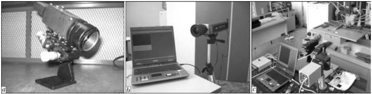
Figure 1. Optical unit of the «Registrator» system (a), high-speed digital camera CENTURIO C100 (b) and lens spectrograph SL100M (c)
