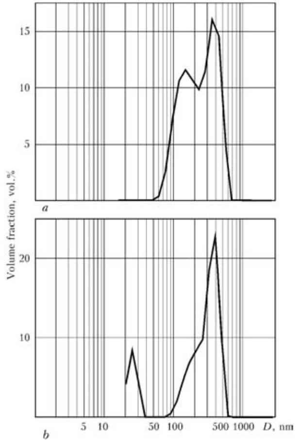
**Figure 3.** Volume distribution of SCWA dispersity of electrodes with coating of rutile MR-3 (a) and basic UONI-13/55 (b) type
