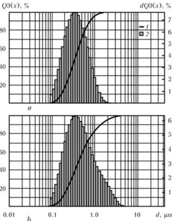
**Figure 2.** Volume distribution  $Q3(x)$  (1) and distribution density  $dQ3(x)$  (2) of dispersity of SCWA of electrodes with coating of basic UONI-13/55 (a) and rutile MR-3 (b) types
