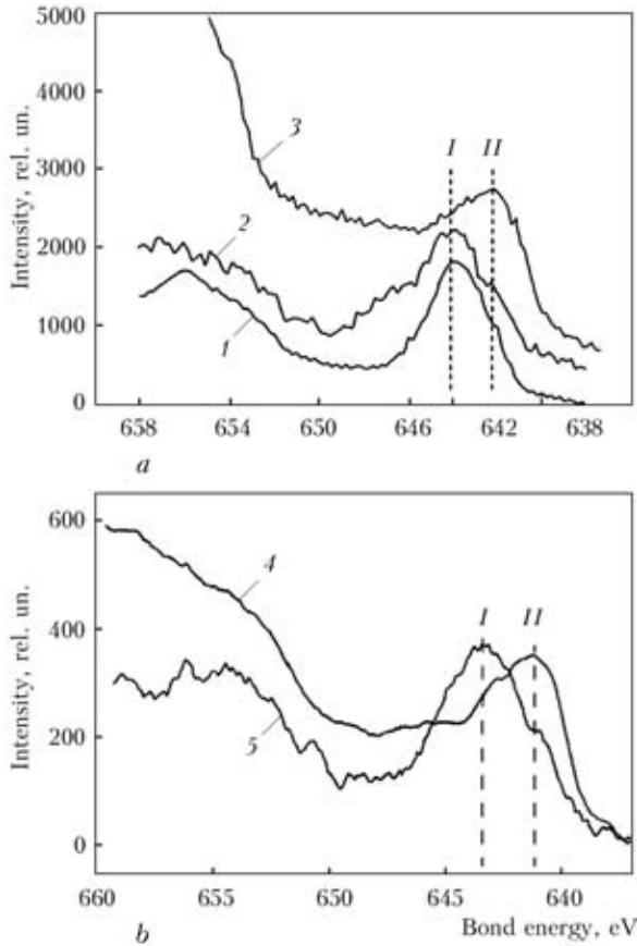
**Figure 1.** Comparison of XPS spectra of SCWA of electrodes with coatings of basic PSh4 (1), PSh5 (2) and rutile E4 (3) types (a) and commercial electrode grades MR-3 (4) and UONI-13/55 (5) (b) (for I, II designations see the text)
