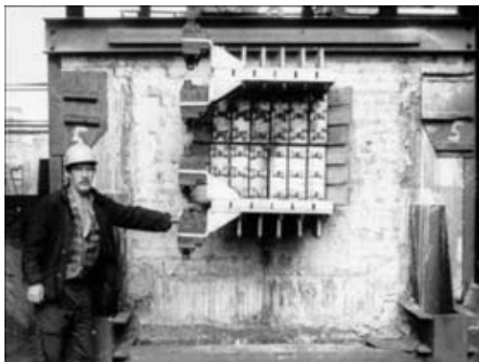
Figure 9. Contact assembly of furnace for carbide silicon synthesis made with ECP application
