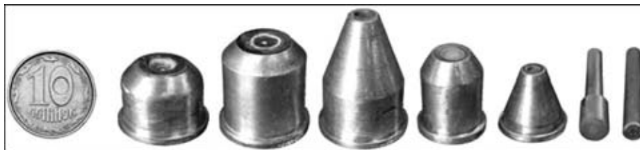
Figure 4. Oxide cathodes of welding arc for different technologies
