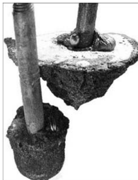
Figure 3. Appearance of the plugs after tear-out test: upper is performed with technology compliance, and lower — with violation
