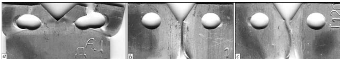
Figure 2. Appearances of fractured specimens of base metal ( a ) and TIG- ( b ) and FS- ( c ) welded joints on alloy AMtsN
