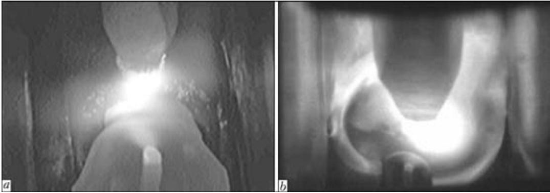
Figure 3. Examples of generated images of TIG welding zone at welding current of 100 (a) and 500 (b) A
