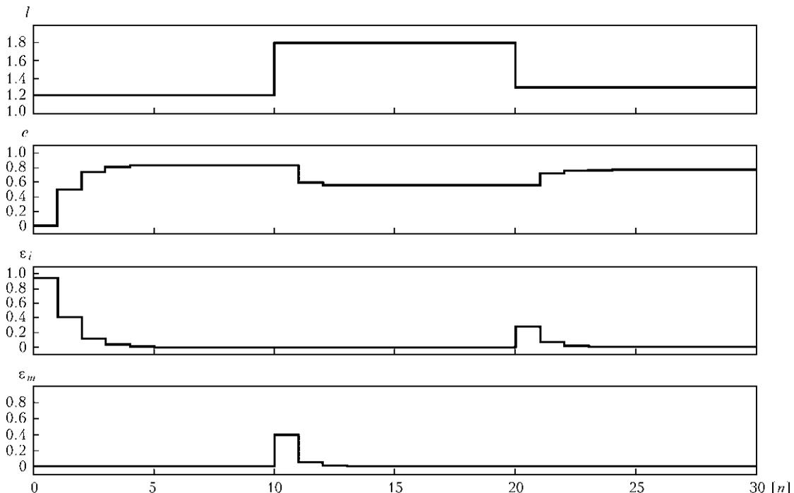
Figure 2. Behaviour of automatic regulator at variation of external lighting of photoreceiver
