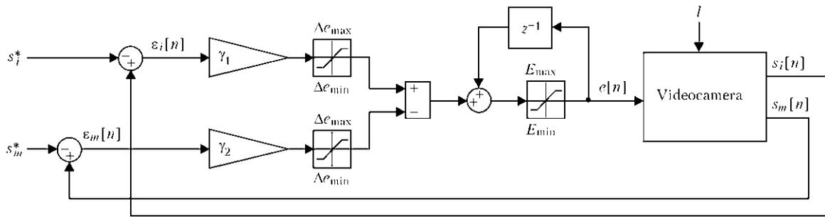
Figure 1. Schematic of automatic regulator for stabilization of image visual quality (for designations see the text)
