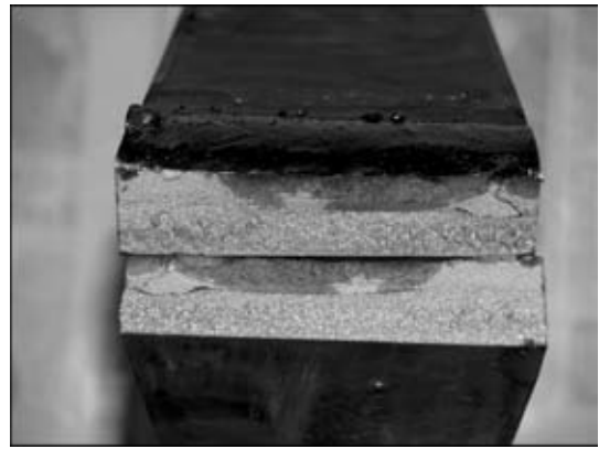
Figure 8. Surface of fracture of welded joint of rail steel with U-groove, made with preheating of up to 250 °C at the heat input of 28.5 kJ/cm after cyclic loading by bending
