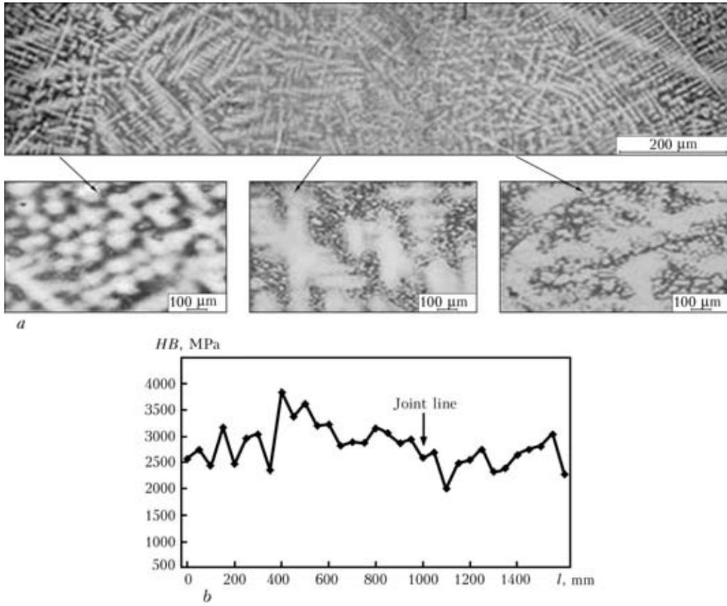
Figure 3. Microstructure (a) and microhardness distribution in the joint of high-temperature alloy produced using nano-structured foil of Ti-Al system (b)
