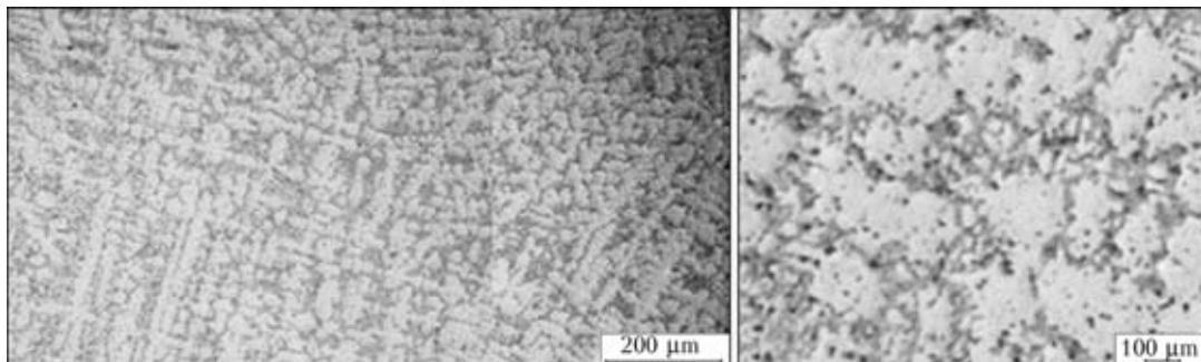
Figure 1. Microstructures of cast high-temperature nickel alloy Rene 80
