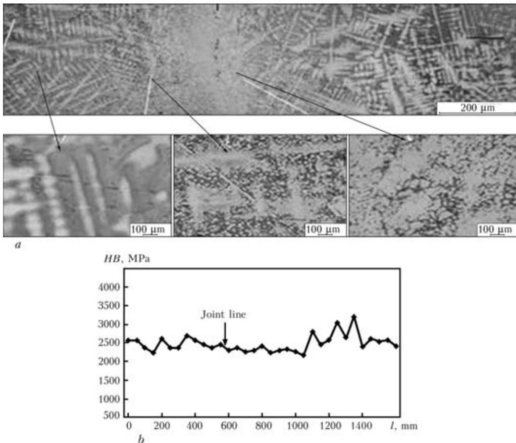
Figure 4. Microstructure (a) and microhardness distribution in the joint of high-temperature alloy produced using nano-structured foil of Ag-Cu system (b)
