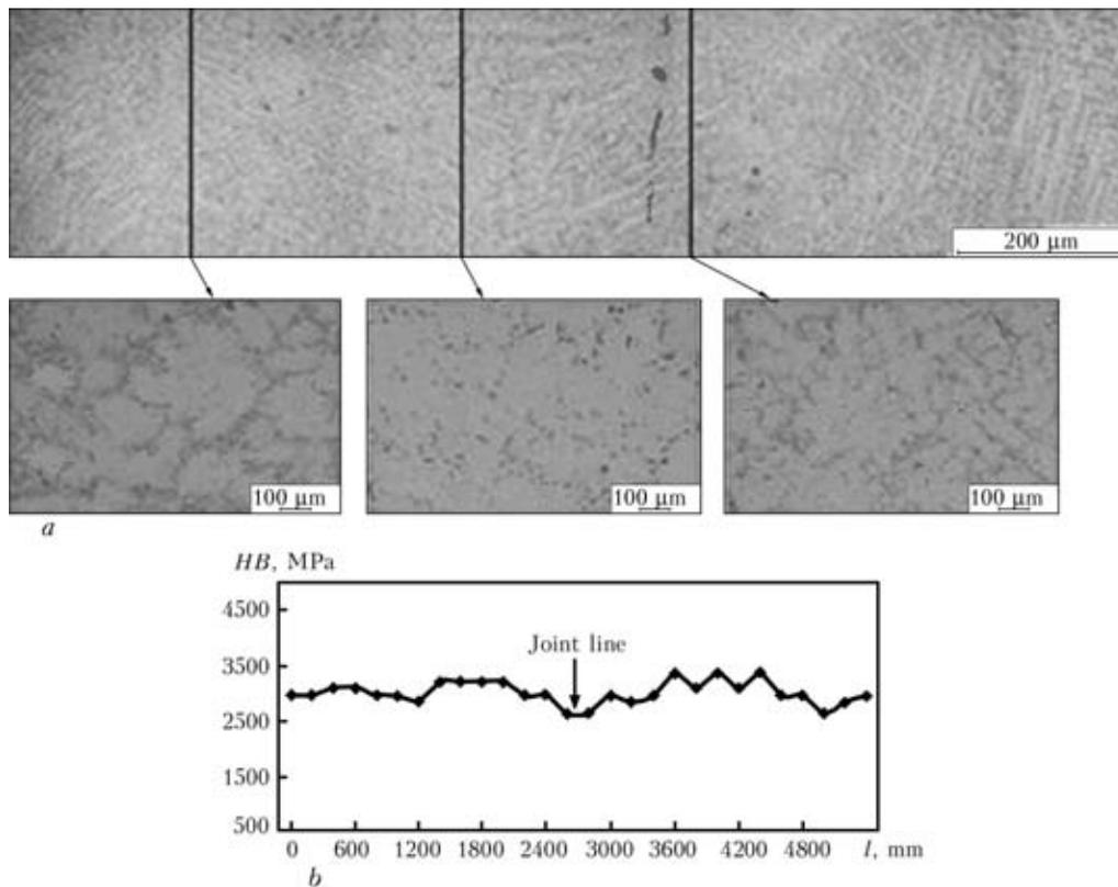
**Figure 2.** Microstructure (*a*) and microhardness distribution in the joint of a high-temperature alloy produced using nano-structured foils (*b*)
