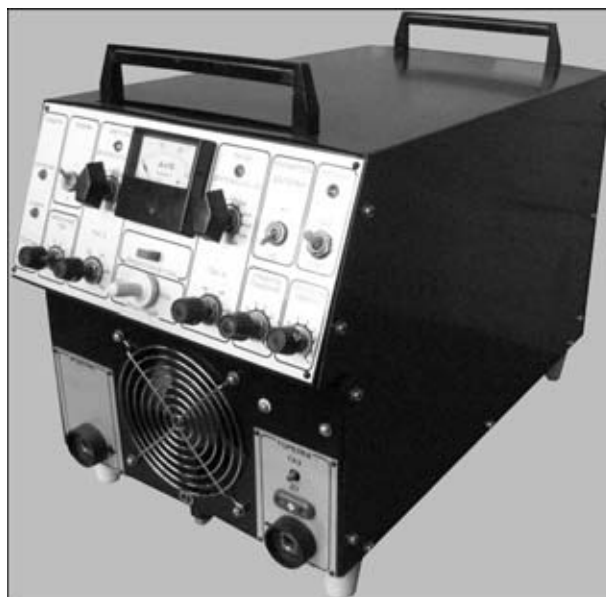
Figure 5. Appearance of welding current regulator RDG-201 UZ.1 for TIG welding
