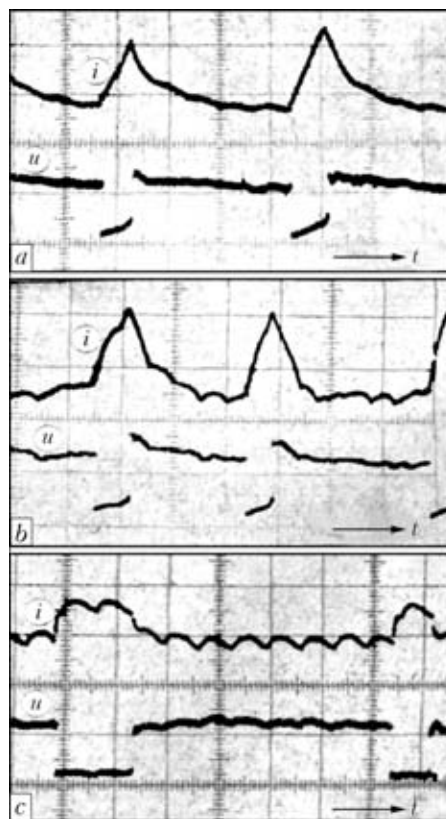
Figure 1. Current and voltage oscillograms with the short-circuit current limited with throttle (a), slope of external characteristic of welding rectifier the transformer of which has a developed scattering (b), and with resistor (c) [2]
