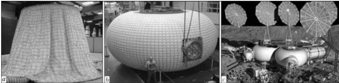
Figure 9. Torroidal Lunar Habitat: a – folded condition; b – completely deployed condition; c – project of NASA manned lunar outpost, constructed on the base of Torroidal Lunar Habitat [6]
