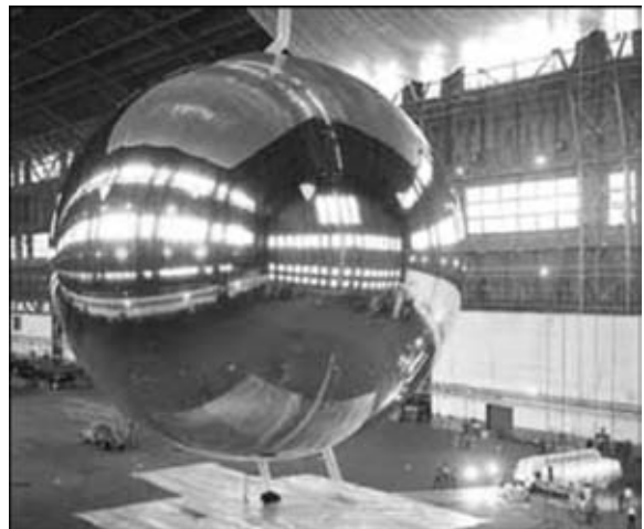
Figure 7. PAGEOS observation satellite with 56 kg mass and 31 m diameter of the shell [8]
