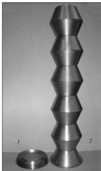
Figure 2. TS of a periodic profile (material – VT1-0 titanium 0.15 mm thick), consisting of 11 basic conical shells [2]: 1 – structure in the compact folded state; 2 – deployed structure
