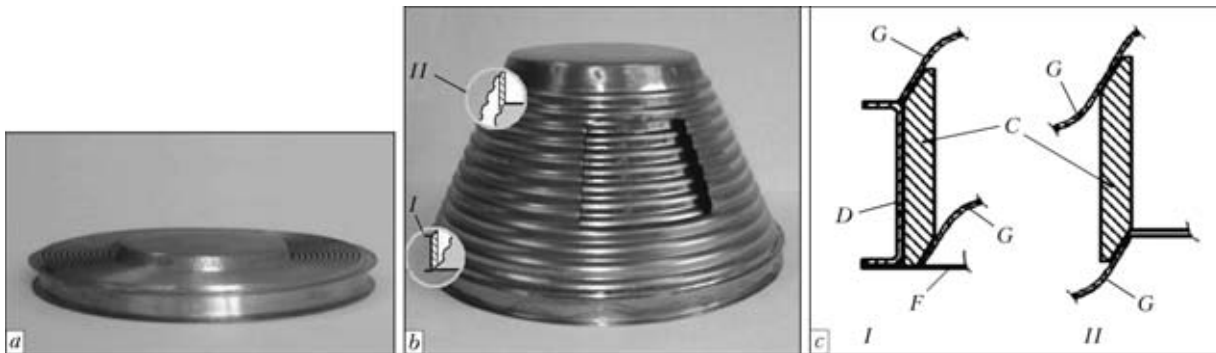
Figure 15. Model of a two-stage transformable conical shell (material – VT1-0 titanium 0.15 mm thick): a – compact condition; b – deployed condition; c – axial sections of load-carrying elements (frame rings) I and II ; C, D – load-carrying and auxiliary frame rings; F – shell bottom; G – transformable conical shells
