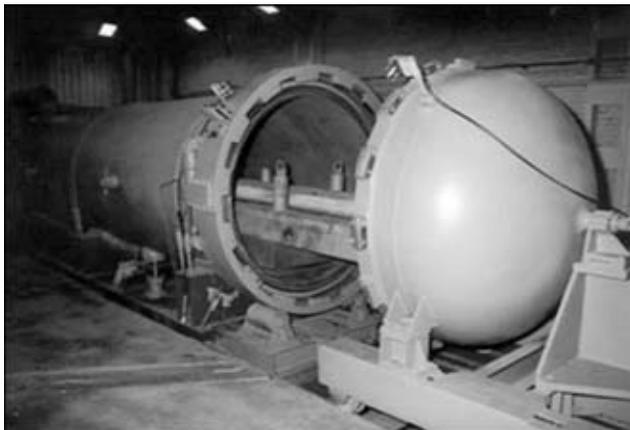
**Figure 1.** Explosion chamber KVG-16 with pulled out work table
