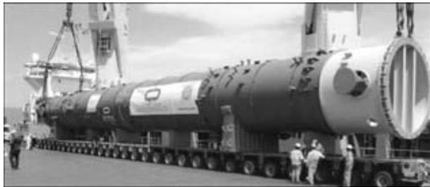
**Figure 9.** Loading of a 500 t slug catcher surge vessel onto a freighter at Gemlik harbour
