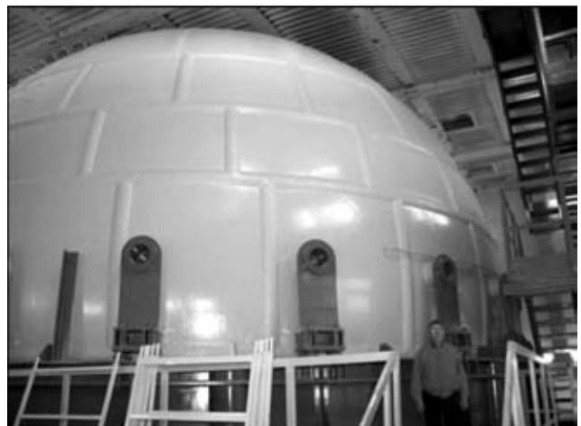
Figure 3. SUEC unique spherical explosion chamber 13YaZ
