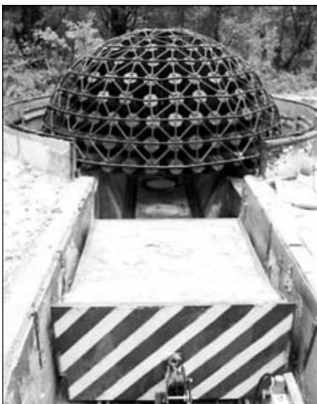
Figure 5. General view of semi-automatic tubular explosion chamber
