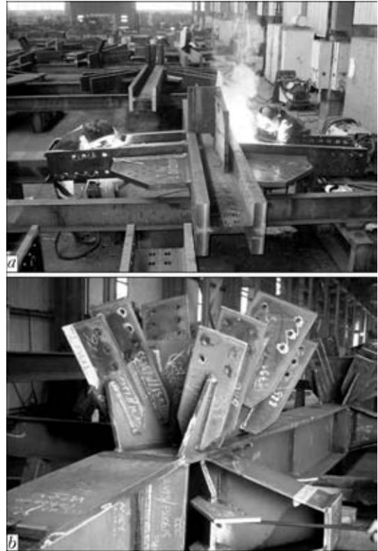
**Figure 8.** Pre-production of the gusset plates for «Eurasia» (a) and «Shakhtar» (b) using flux-cored GMAW in Gemlik
