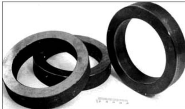
**Figure 1.** Appearance of rings with deposited layer for heat resistance tests
