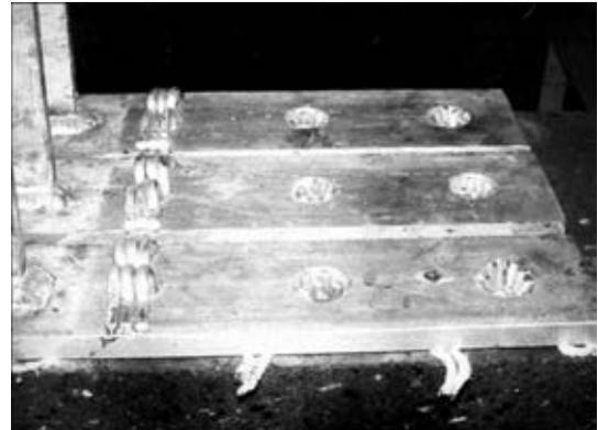
**Figure 10.** Element of contact assembly of Acheson furnace prepared for erection welding
