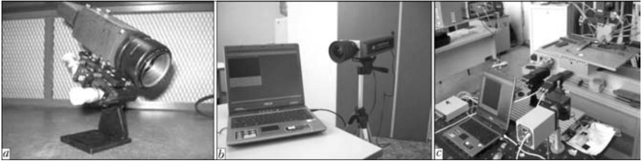
Figure 1. Optical unit of the «Registrator» system (a), high-speed digital camera CENTURIO C100 (b) and lens spectrograph SL100M (c)
