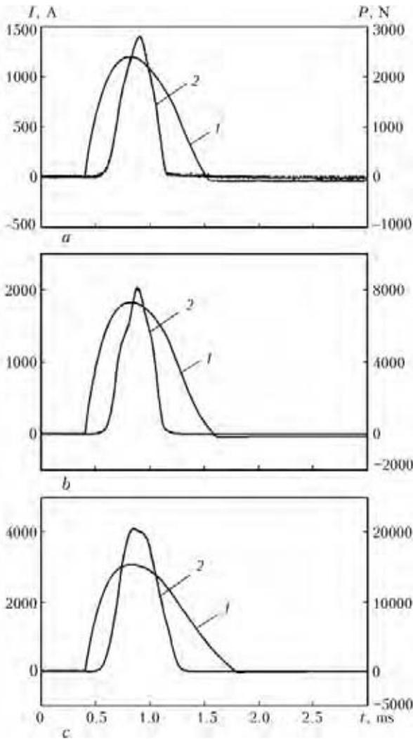
**Figure 5.** Amplitude values of pulsed current  $I$  (1) and dynamic load  $P$  (2) at different values of charge voltage:  $a - U = 200$  V,  $I_{\max} = 1195$  A,  $P_{\max} = 2792$  N;  $b - U = 300$  V,  $I_{\max} = 1838$  A,  $P_{\max} = 8162$  N;  $c - U = 500$  V,  $I_{\max} = 3080$  A,  $P_{\max} = 20461$  N
