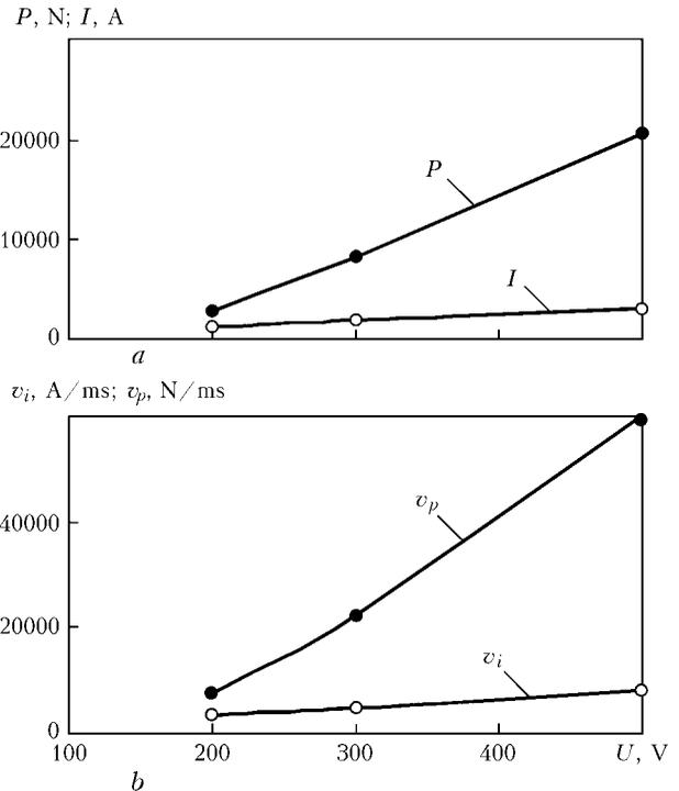
**Figure 6.** Effect of charge voltage  $U$  on pulsed current  $I$ , dynamic loading  $P$  (a) and rate of their growth  $v_i$  and  $v_p$  (b)
