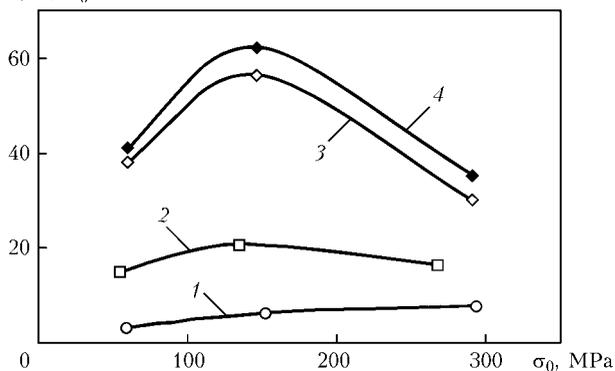
**Figure 3.** Effect of initial stress  $\sigma_0$  on relative efficiency  $\Delta\sigma/\sigma_0$  at EDT of alloy AMg6 and its welded joints at different values of charge voltage: 1 –  $U = 200$ ; 2 – 300; 3, 4 – 500 V; 1–3 – base metal; 4 – welded joint
