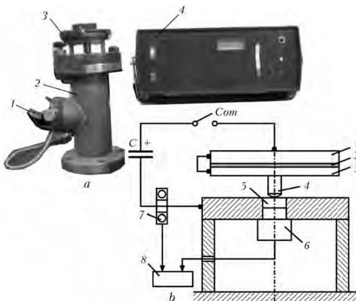
**Figure 4.** Appearance of hardware complex for measuring amplitude values of pulsed current  $I$  and dynamic loading  $P$  at EDT (*a*: 1 – Rogowski loop; 2 – casing of system for measuring load  $P$ ; 3 – inductance coil with electrode; 4 – unit of charge and discharge of capacitors) and its design diagram (*b*) (for 1–8 see the text)
