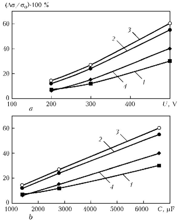
**Figure 2.** Effect of charge voltage  $U$  (*a*) and capacitance of battery of capacitors  $C$  (*b*) on relative efficiency of EDT  $(\Delta\sigma/\sigma_0) \cdot 100 \%$  of alloy AMg6 and its welded joints at different values of initial stress: 1 –  $\sigma_0 = 55$ ; 2, 3 – 130; 4 – 270 MPa; 1, 2, 4 – base metal; 3 – welded joint
