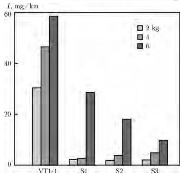
Figure 5. Intensity  $I$  of wear of specimens versus load
