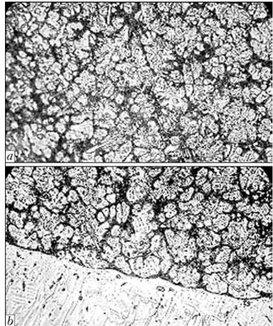
**Figure 3.** Microstructure ( $\times 200$ ) of central part of deposited metal layer (*a*) and fusion zone (*b*)
