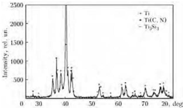
Figure 4. Typical X-ray pattern of metal of the layer deposited on the VT1-1 substrate
