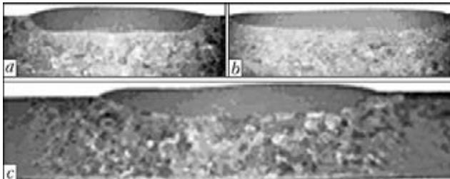
**Figure 1.** Effect of values of magnetic induction on width of deposited layers: *a* –  $B = 6.2$  (S1); *b* – 7 (S2); *c* – 7.5 mT (S3)
