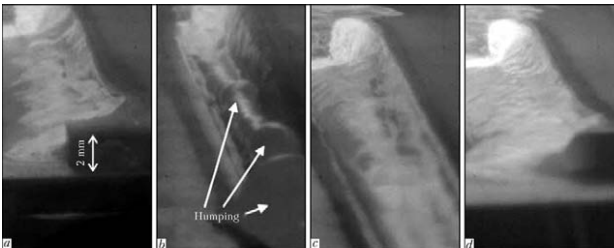
Figure 9. Influence of shielding gas on humps formation in overlap joint (steel S420MC 2 mm thick, v_w = 10 m/min, shots behind the welding process): a, b – without shielding gas; c, d – with Ar + O 2 gas
