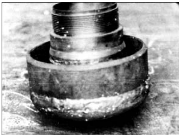
Figure 2. Appearance of a lance after welding of copper snout to steel ring
