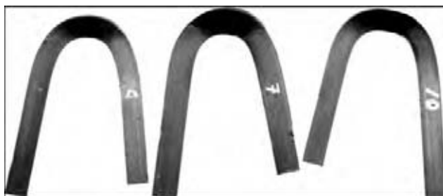
Figure 7. Appearance of copper to steel welded specimens after bend tests
