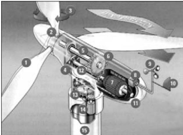
**Figure 1.** Schematic of a wind generator: 1 – blades; 2 – rotor; 3 – system of blade rotation in rotor bushing; 4 – system of deceleration of rotor rotation; 5 – drive shaft with low speed of rotation; 6 – transmission; 7 – generator; 8 – control system; 9 – wind speed measuring instrument; 10 – system of wind direction monitoring; 11 – nacelle; 12 – shaft with high rotation speed; 13, 14 – drive and motor of nacelle rotation system; 15 – tower
