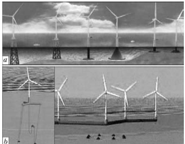
**Figure 4.** Constructions of wind generators with their base in the sea coastal strip (*a*) and floating ones (*b*)
