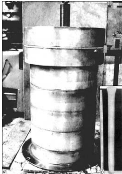
Figure 9. Appearance of welded shell with changeable thickness of wall made of AMg6 alloy forgings (a), and macrosection of joint (b)
