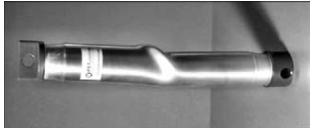
Figure 10. Sample of MP-welded main shaft (aluminum-steel) after successful strength tests in torsion
