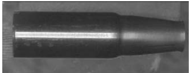
Figure 11. Fragment of sample of MP-welded fuel slug
