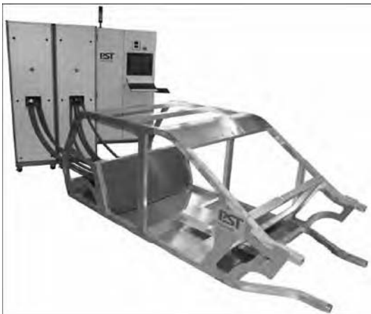
Figure 3. First in the world lightweight frame of car body from dissimilar metals, wholly manufactured using MPW
