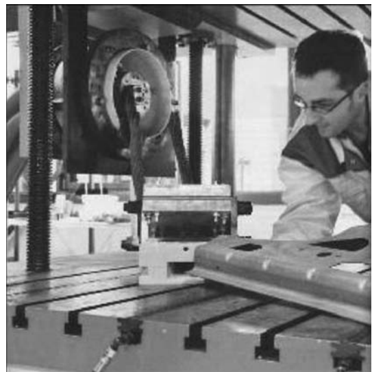
Figure 12. Magnetic-pulse cutting (punching) of parts of automobile designation using elements of PST equipment in Fraunhofer IWU [28]
