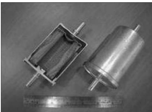
Figure 9. Fuel filter manufactured using MPW
