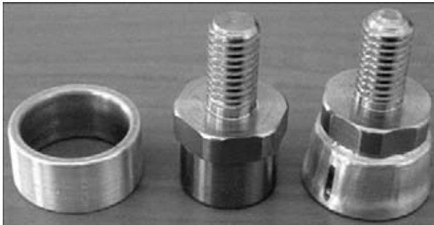
Figure 8. Aluminum ring MP-welded to steel bolt
