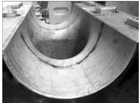
Figure 6. Die block for forming of large-diameter three-way pipes after plasma hardening
