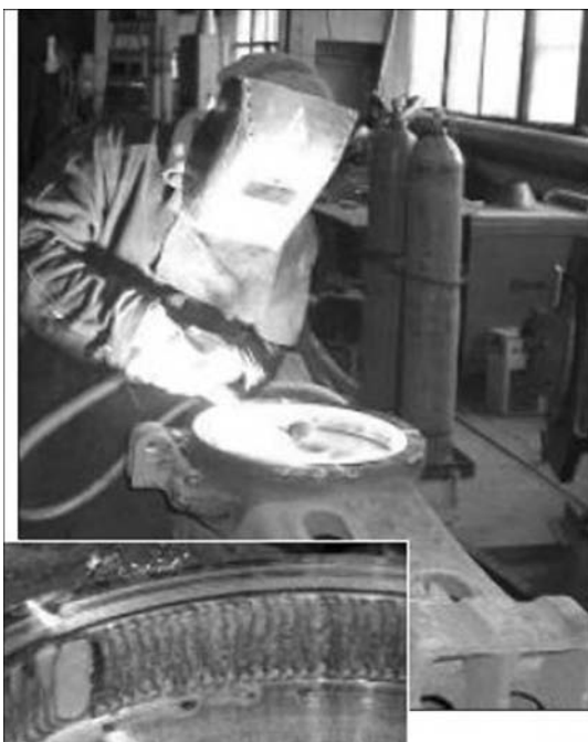
Figure 8. Plasma hardening of freight car centre plate collar and fragment of hardened surface
