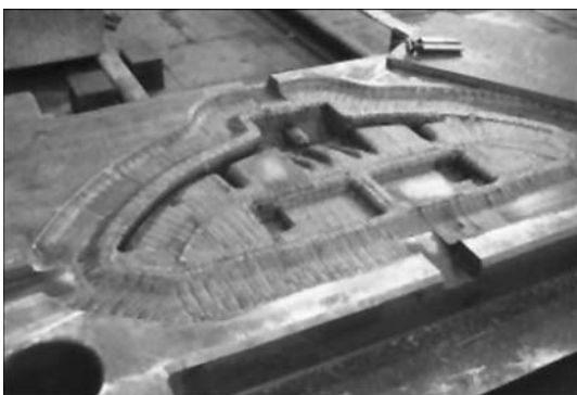
Figure 3. Complex-configuration die after plasma hardening (KUMZ Ltd.)
