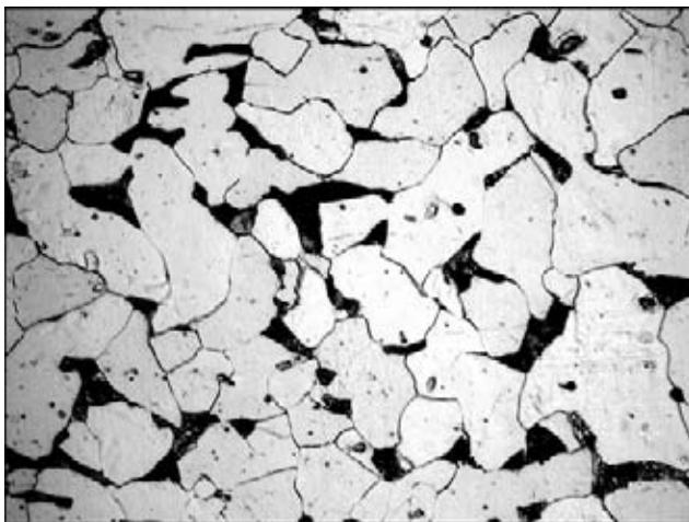
Figure 1. Microstructure (x500) of steel VSt3sp
