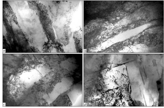
**Figure 7.** Changes in fine structure of heat-treated (T = 350 °C, t = 1 h) weld metal on alloy 1460 under conditions of dynamic loading depending on the alloying method (without and with scandium): a, b — intensive SBs in metal without scandium (×20,000 and ×30,000, respectively); c, d — fragmentation of structure due to blocking of SBs by the scandium phases in Sc-containing metal (×30,000)
