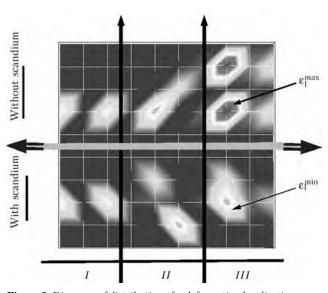
**Figure 6.** Diagrams of distribution of  $\varepsilon_l$  deformation localization zones in the 1460 alloy weld metal obtained by using filler wires Sv1201 and Sv1201 + Sc in the as-welded state (*I*) and after heat treatment at *T* = 150 °C, *t* = 22 h (*II*) and at *T* = 350 °C, *t* = 1 h (*III*)
