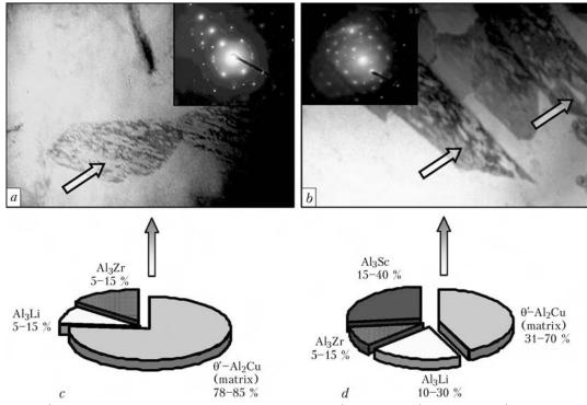
**Figure 9.** Changes (under heat treatment conditions at T = 350 °C, t = 1 h) in structure (a, b - x50,000) and composition (c, d) of  $\theta$ '-phase formations in weld metal of the welded joint on alloy 1460 depending on the method of alloying without (a, c) and with (b, d) scandium
