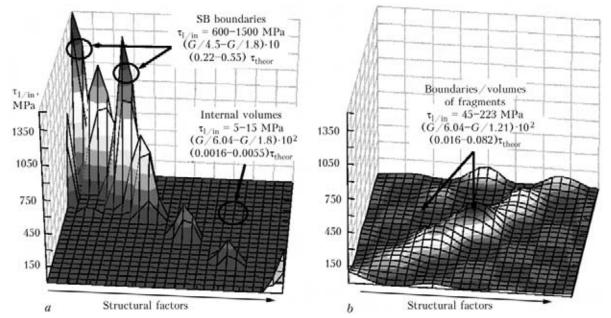
**Figure 8.** Distribution of local internal stresses  $\tau_{1/in}$  in weld metal of the Sv1201 (*a*) and Sv1201 + 0.5 % Sc (*b*) types (heat treatment at T = 350 °C, t = 1 h) after external dynamic loading
