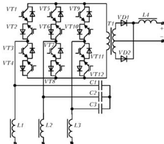
Figure 2. Elementary diagram of power components (acc. to Figure 1)
