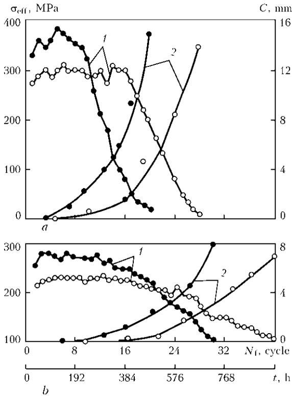
**Figure 4.** Fracture diagrams of welded joints on steel 12Kh18N12T at  $\epsilon_a = 0.5$  (a) and 0.2 (b) %: 1 –  $\sigma_{eff} = f(N_f)$ ; 2 –  $C = \varphi(N)$ ; dark circles – as-welded state; light circles – after austenising
