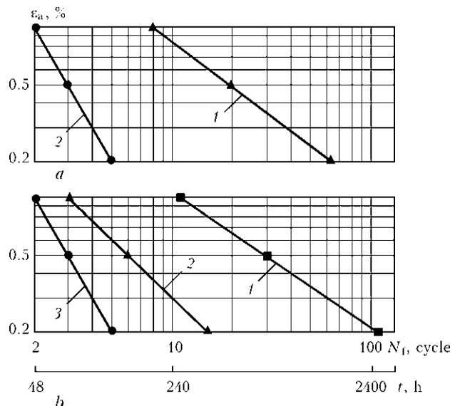
**Figure 3.** Effect of notch sharpness (theoretical stress concentration factor) on long-time low-cycle strength of welded joints on steel 12Kh18N12T in the as-welded state (*a*) and after austenising (*b*) at  $T = 823$  K and  $\nu = 4.2 \cdot 10^{-2}$  cycle/h: *1* – without notch; *2* – Mesnager type notch (3.0); *3* – Charpy type notch (5.3); *t* – total test time
