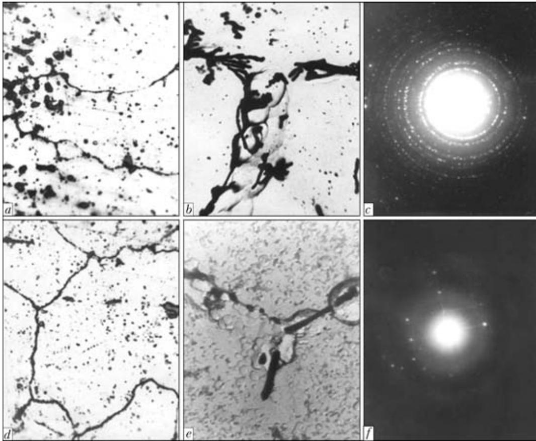
**Figure 2.** Microstructures of HAZ metal on steel 12Kh18N12T at different distances from the weld and at different magnifications (*a, d* –  $\times 700$ ; *b, e* –  $\times 5000$ ): *a, b* – fusion line; *d, e* – 0.1 mm from the fusion line; *c, f* – electron diffraction patterns of the carbide phase of TiC and Cr<sub>23</sub>C<sub>6</sub> compositions, respectively
