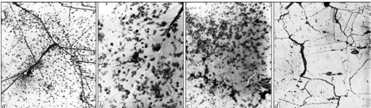
**Figure 5.** Microstructures of HAZ metal after the low-frequency low-cycle loading tests ( $\epsilon_a = 0.5$  %,  $\tau_l = 24$  h and  $T = 823$  K): a – formation of discontinuity at a junction of three grains ( $\times 1000$ ); b, c – precipitation of carbide phase in structure of TiC ( $\times 5000$ ); d – network of wedge-shaped cracks ( $\times 300$ )
