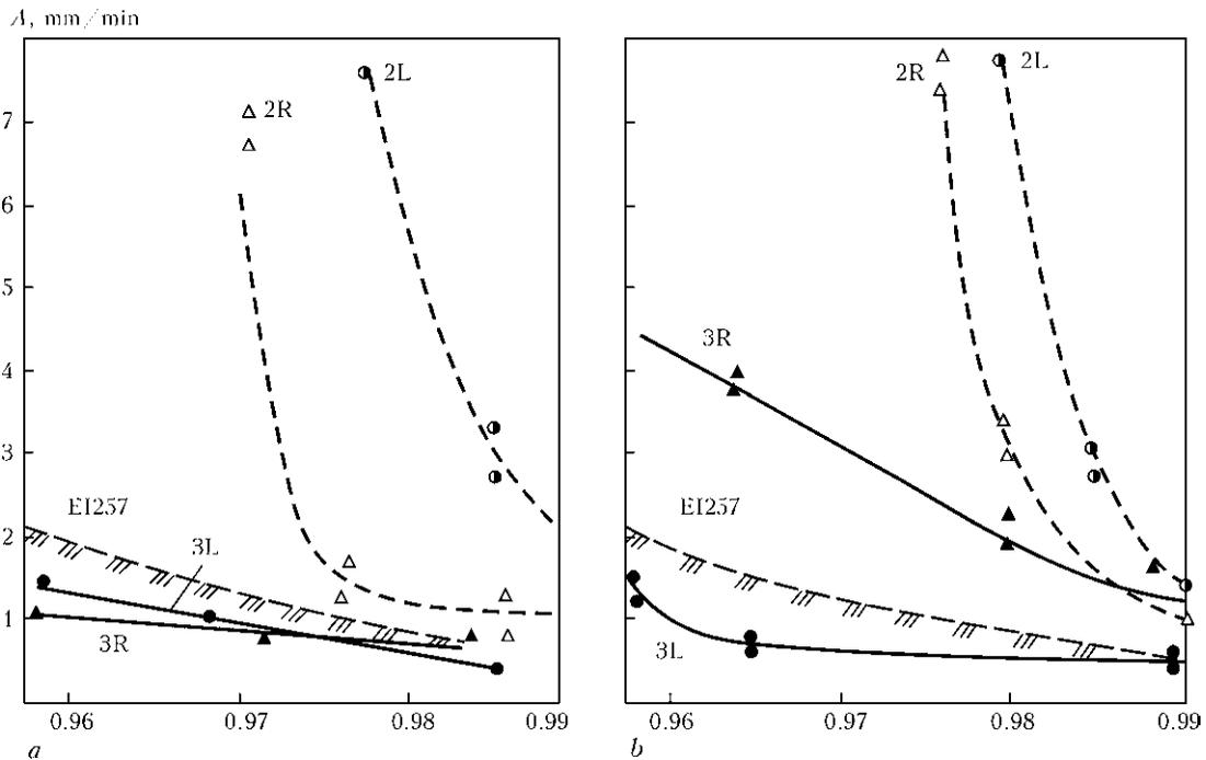
**Figure 1.** Resistance of steels 12Kh18N12T and EI257 to formation of hot sub-solidus cracks in HAZ metal in a state after operation (a), overheating and austenising at 1373 K (b): 2R, 2L, 3R, 3L – metal of the pipes adjoining the welds of joints 26L and 3A on their right and left sides (values of relative temperature  $\theta$  are marked on the axis of abscissa)
