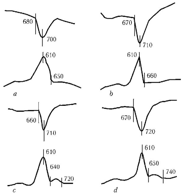
**Figure 1.** Data of differential thermal analysis of the alloys: a – Ag-Cu-Zn-Ni-Mn (amorphous foil); b – Ag-Cu-Zn-Ni-Mn (cast); c – Ag-Cu-Zn-Mn-2Pd; d – Ag-Cu-Zn-Ni-Mn-5Pd
