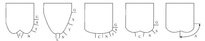
Figure 4. Schematics and codes of wear of cutting structure of bits: N - cutting structure that is closest to the bit top (middle row of bit cutters M is located between rows N and G); G - gauge row, cutting structure located on the gauge surface of bit; A - all rows (entire cutting structure of bit); C - inside cone surface; T - outside cone surface; S - shoulder
