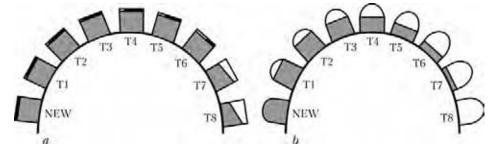
**Figure 2.** Schematic of wear of DHACs (a) and hard-alloy inserts (b): a: 0 – bit cutter is not worn out; 1-7 – cutter is worn out to 10, 15, 25, 30, 50, 70 and 100 %, respectively; 8 – complete loss of cutting structure; b: 0 – bit insert is not worn out; 2, 4, 6 – insert is worn out to 25, 50 and 75 %, respectively
