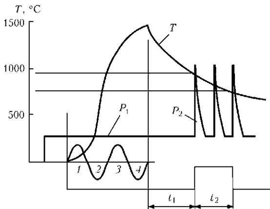
**Figure 2.** Cyclogram of the process of braze-welding with impact application of the peening force
