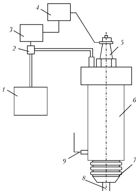
Figure 1. Schematic of the drive of electrode assembly for spot braze-welding (for 1-9 see the text)
