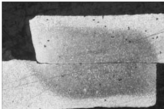
**Figure 5.** Typical macrosection ( $\times 50$ ) of brazed joint with impact peening of the joint zone
