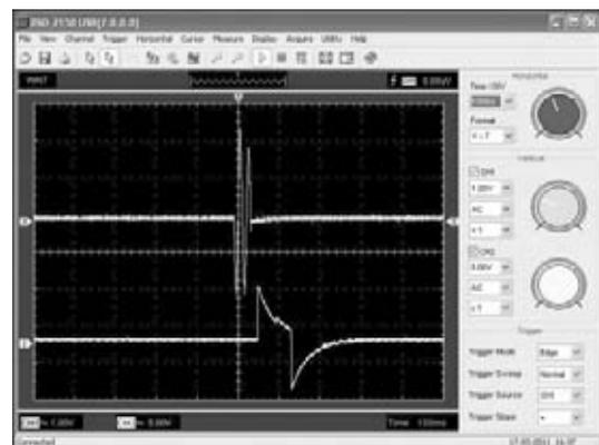
**Figure 4.** Oscillogram of welding current pulses and current pulses in the circuit of explosive application of the compressive force
