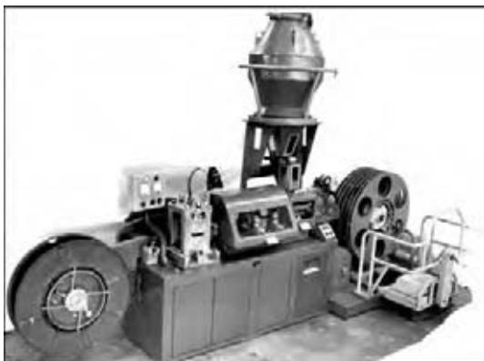
**Figure 6.** Mill OB 2324 for manufacture of single-lock flux-cored strip with tight lock
